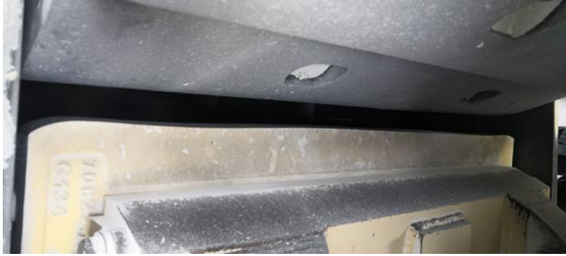
Figure 8. Blow bar gap and profile after utilization.
